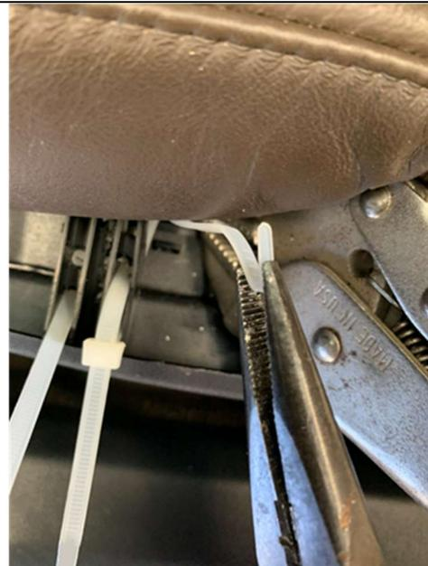
Here you can see both ends of the zip ties before I feed the ends through and tighten them
