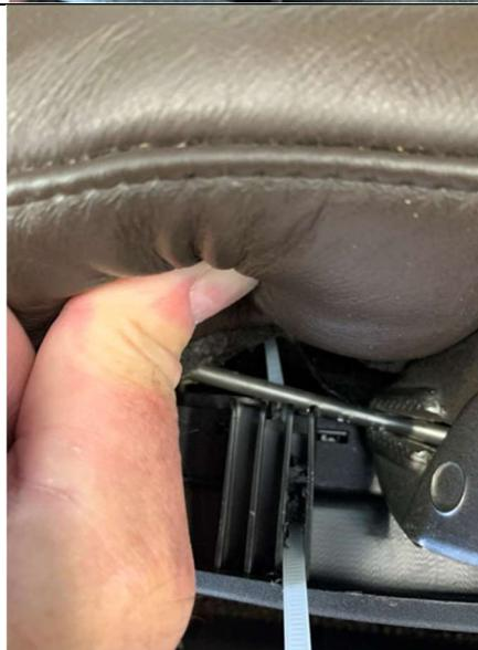
I repeated the holes in the other channel on the clip to ensure the ties held for the long term. If one is good, two are better!
