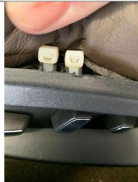
Here is where you pull the ties tight as possible. I held them with the needle nose pliers and pulled them tight with another set of pliers then clipped off the ends.
