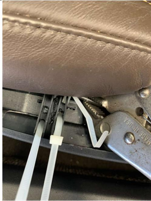
Use your needle nose pliers and bend the end of the zip tie so there is a good 90 degree bend in the end this helps feed the tie up through the drilled hole.
