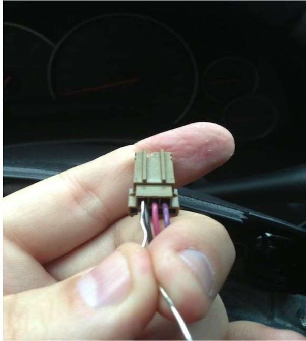
To reassemble -- reverse your steps. Connect the right paddle to its wire connector and mount it with the two #20 Torx (if removed.) Replace the cover with one #20 Torx.
