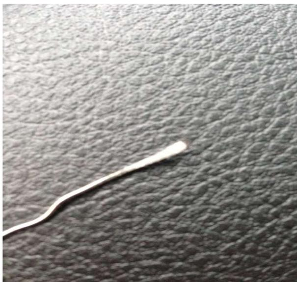
Then insert the paper clip in the back of the connector on top of the wire. Don't pay attention to the color code in my picture because I didn't take it till the swap was already done. When the paper clip is inserted correctly the wire will slide right out. Its hard to explain but you can kind of feel a pop when its correct. Don't pull on the wire until the paper clip is inserted because that will make it harder to come out.
