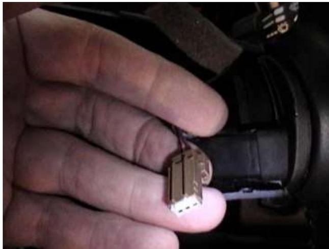
I then opened up the connector by sliding the white retaining clip out by pressing in on the sides. Here's a close up showing the wires (brown/tan, pink, purple.)
