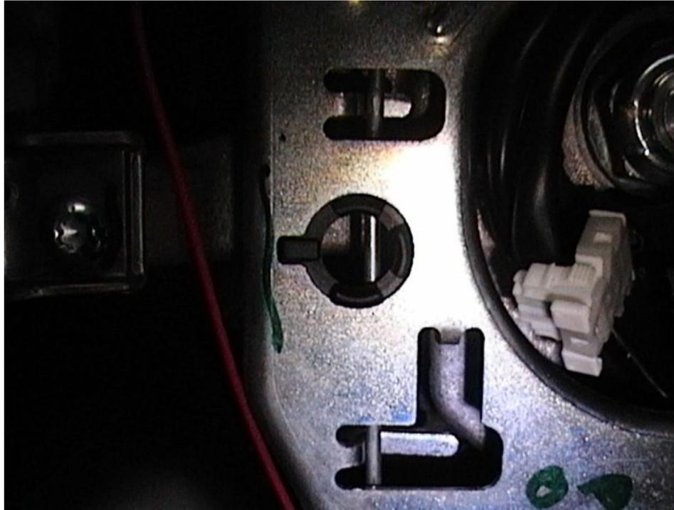
The next photo below shows the spring-wire pushed back that allows the airbag to pull out. You can see the punch inserted.
