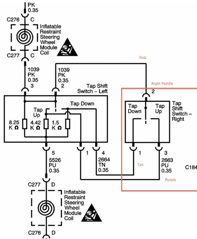
First thing, for your own safety disable the airbag in the steering wheel. I disconnected the ground wire. It is next to the fuse box in the engine bay and takes a deep-well 13mm socket. Wait at least 10 minutes before working with the airbag.
