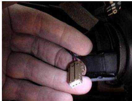
I then opened up the connector by sliding the white retaining clip out by pressing in on the sides. Here's a close up showing the wires (brown/tan, pink, purple.)
