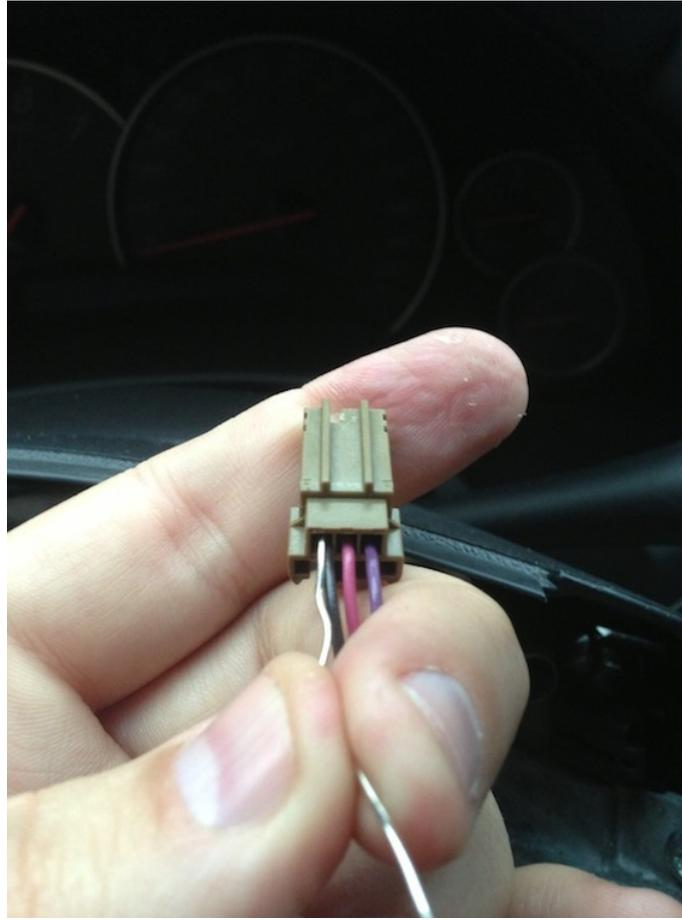
To reassemble -- reverse your steps. Connect the right paddle to its wire connector and mount it with the two #20 Torx (if removed.) Replace the cover with one #20 Torx.
