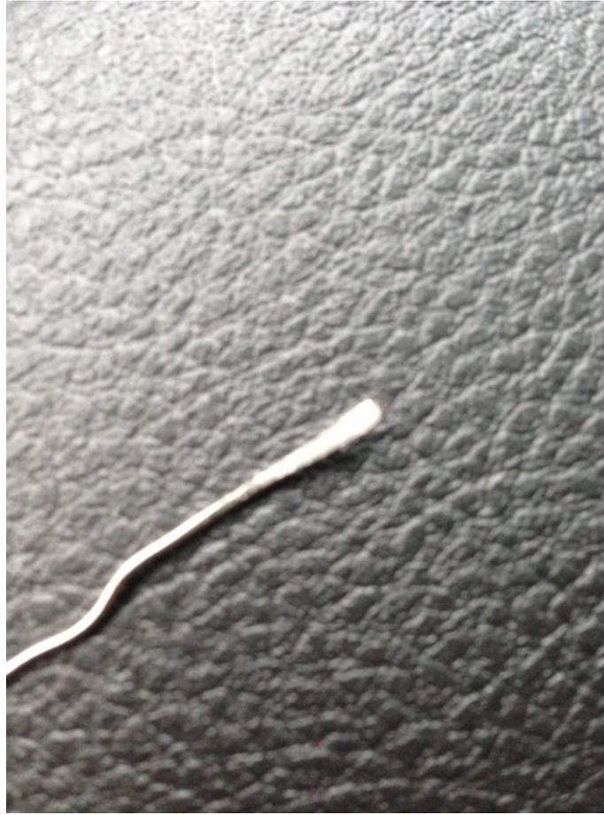
Then insert the paper clip in the back of the connector on top of the wire. Don't pay attention to the color code in my picture because I didn't take it till the swap was already done. When the paper clip is inserted correctly the wire will slide right out. Its hard to explain but you can kind of feel a pop when its correct. Don't pull on the wire until the paper clip is inserted because that will make it harder to come out.
