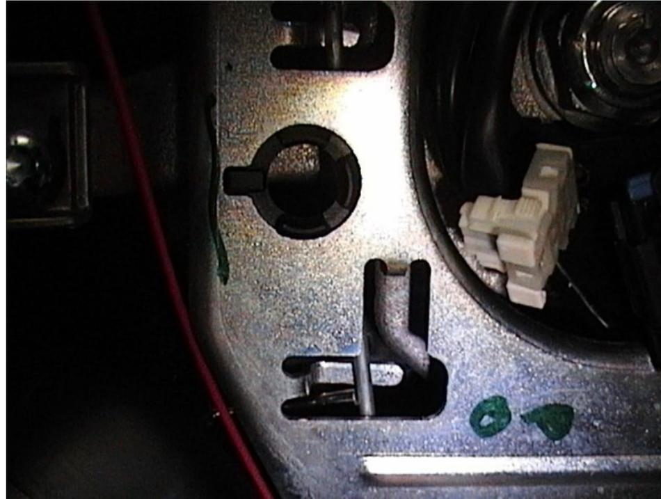
Pull the airbag toward you as you press the spring-wire and it will release as shown below.
